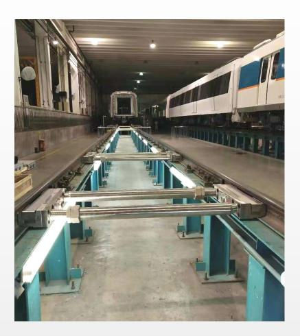
It is a load cell based system, which fits to the inner sides of rail. When the wheel flange rolls up the ramp, the wheel's tyre is raised, so the wheel-rail contact force is tested on the wheel flange.
